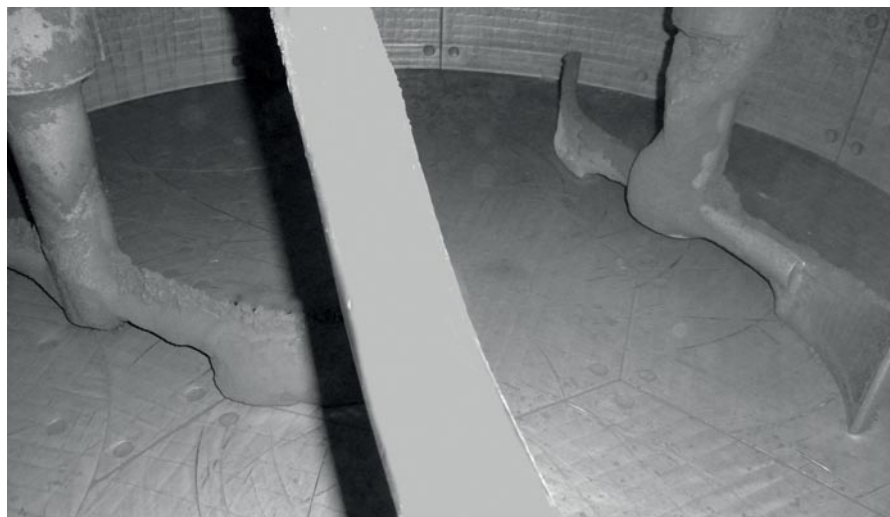
Depending on the size of the mixer the use of several mixing turbines is also possible, even when converting existing planetary mixers
