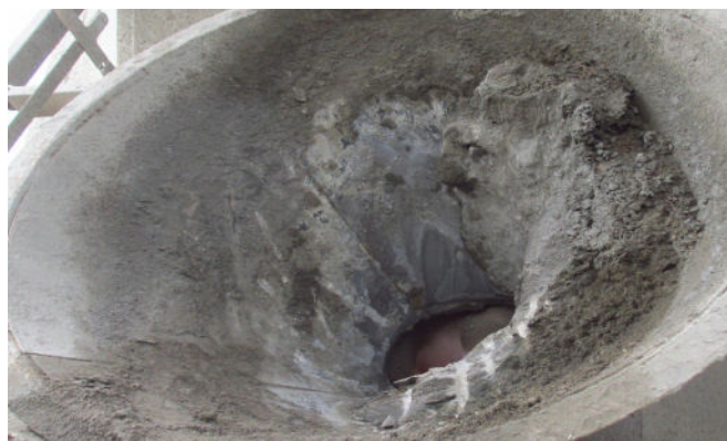
Typical example of build up in steel discharge chute
