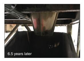
Our Solution: ConeFlex abrasion-resistant conical chute liner
