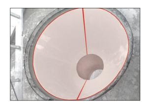
Our Solution: Hawiflex® ConeFlex conical discharge chute liner
