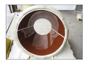
Our Solution: Hawiflex® EasiFix polyurethane lining with foam rubber backing
