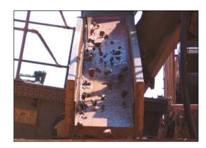
Our Solution: Hawiflex® EasiFix polyurethane lining with integral foam backing
