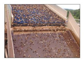
Our Solution: Hawiflex® polyurethane sheet - 10mm thick
