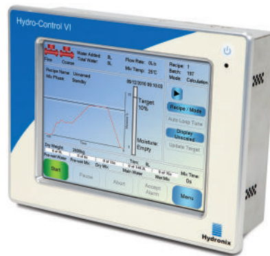
Hydronix Hydro-Control VI automatic water control system
