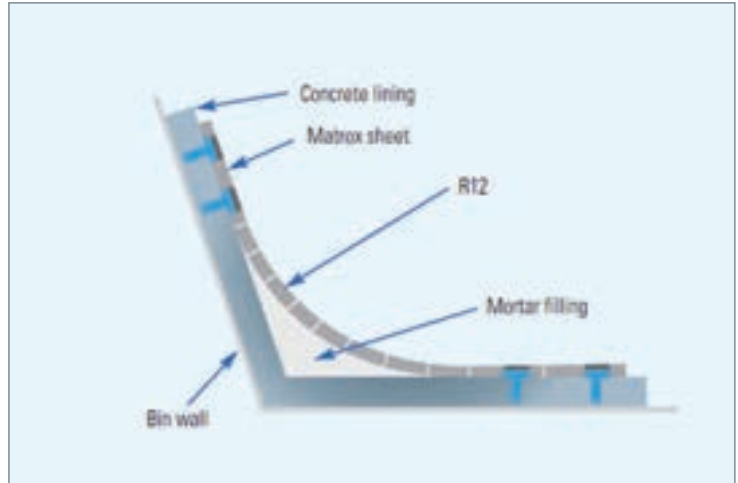
Fastening of hopper lining
