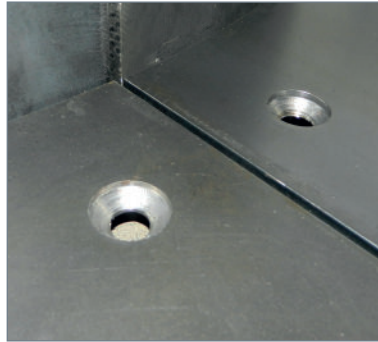
Holes countersunk to optimum depth
