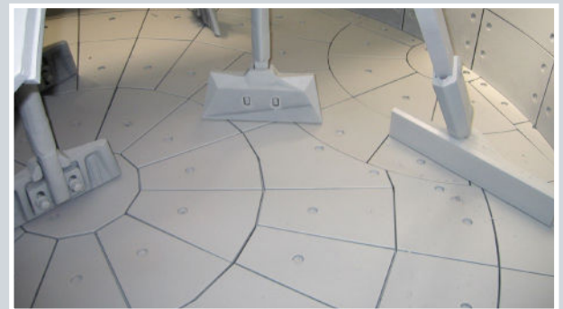
Chill Cast Tiles: Maximum abrasion resistance
