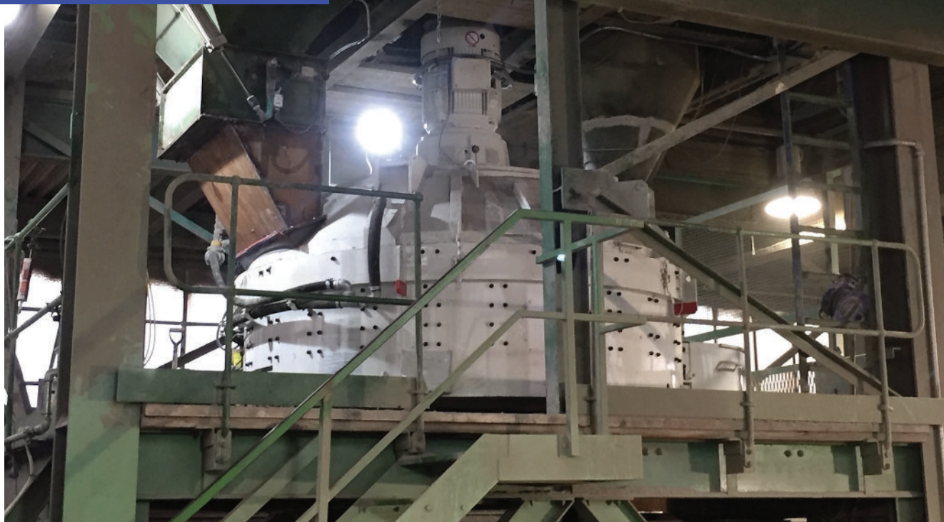
One of Besblock's new TEKA planetary mixers, supplied and installed by ConSpare
