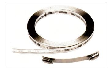
The connectors use 'straight line' housings which ensure that every thread of the screw is fully engaged with the band. This special feature, together with a high tensile band and hardened rolled thread screws, means that our clamp bands have more than twice the strength of ordinary worm drive hose clips.
