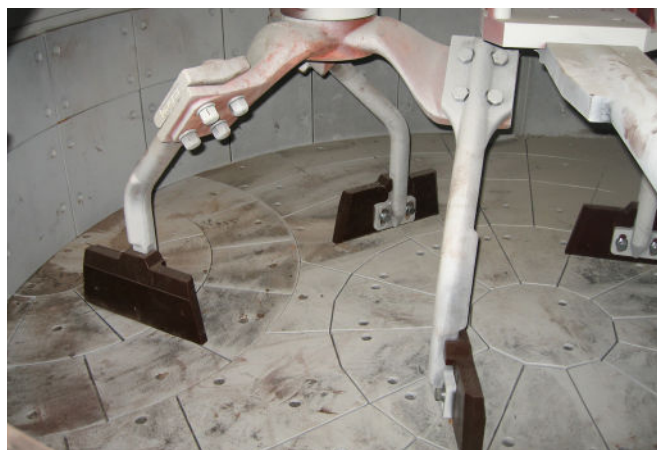
Counter-current mixing stars give high efficiency mixing
