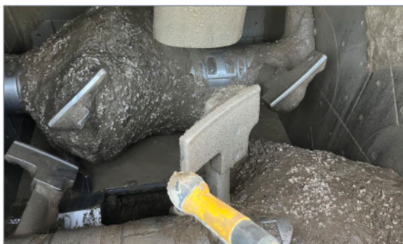
Example of concrete build-up on the mixer shafts and mixing arms
