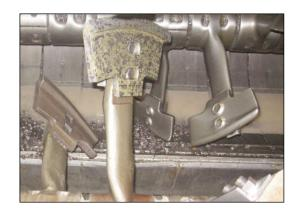
Our Solution: Ultra Tungsten carbide protected mixing blade
