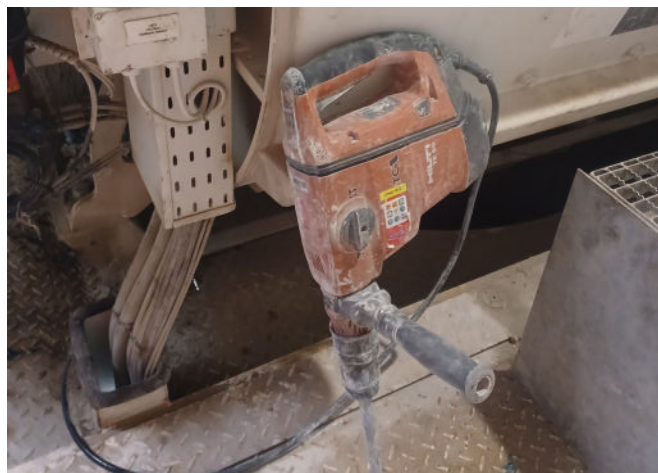
The 110V electric breaker previously used 4-5 hours a week
