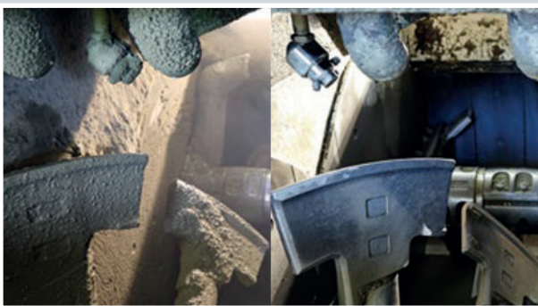
Before and after: 10 minute automated high pressure cleaning cycle
