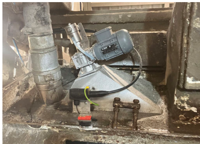
Head mounting customised to optimise cleaning pattern
