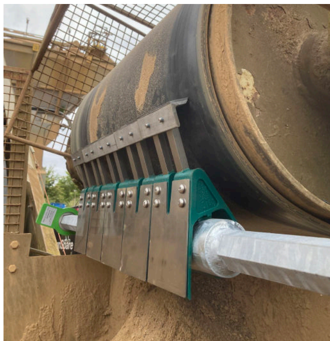
STARCLEAN® primary cleaner with tungsten carbide blades
