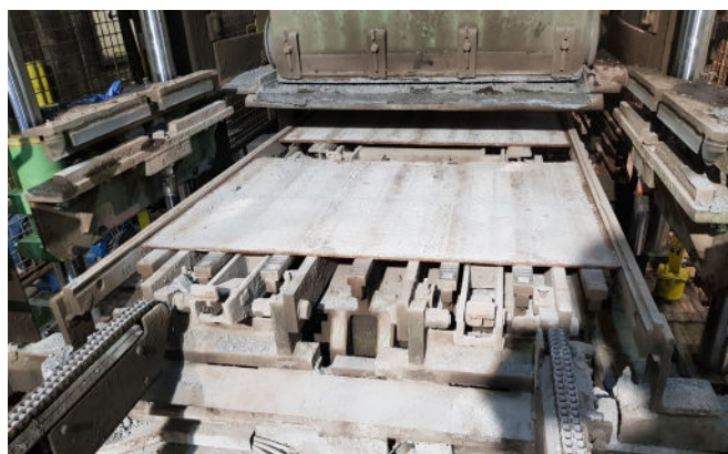
Block machine vibration table at client's factory
