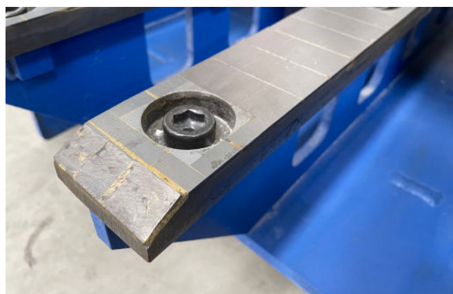
Special tungsten carbide segments developed for application
