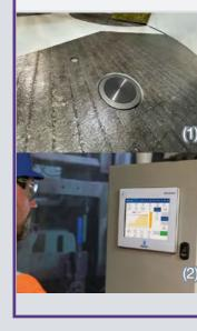
Accurately measuring moisture in the mixer optimises the entire mixing and production process.
