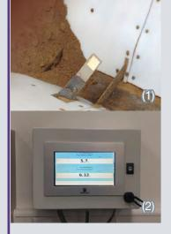
Moisture in sand and aggregates is the hidden variable in the process. Failure to identify this water content has a significant effect on the cost of production, the carbon footprint of the plant, and product quality.
