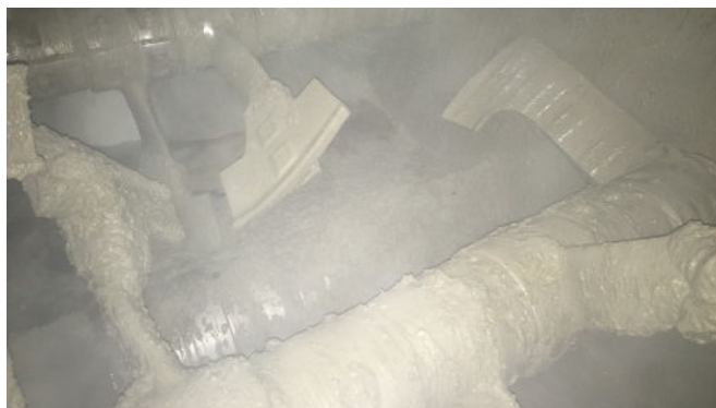
Concrete regularly building-up in the twinshaft mixer
