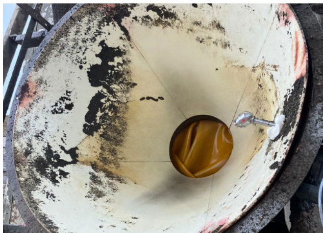
Automated cleaning of the ConeFlex discharge chute
