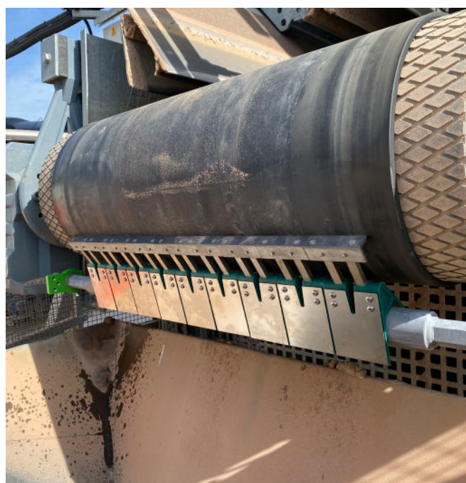
STARCLEAN® belt cleaner with 14mm of tungsten on blades
