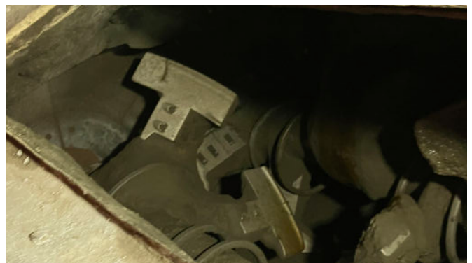
Mixer cleaned with hand lance alone - full of build-up
